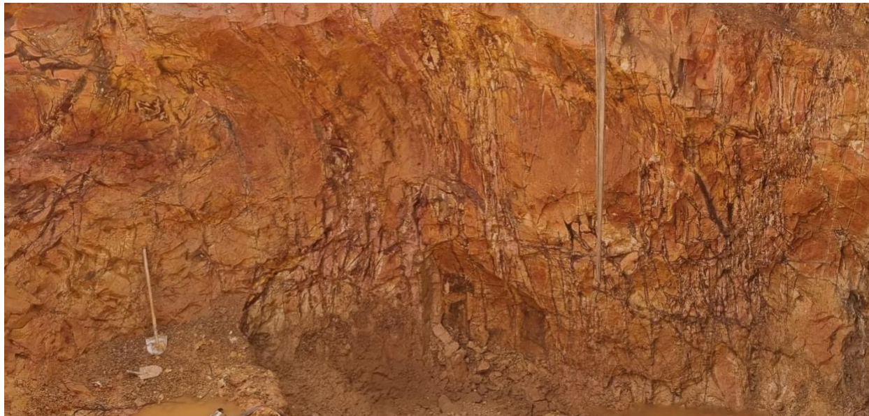
Figure 2: Example of stockwork-like intersecting vein arrays hosted in saprolitic greywacke at Daina 1 South.
